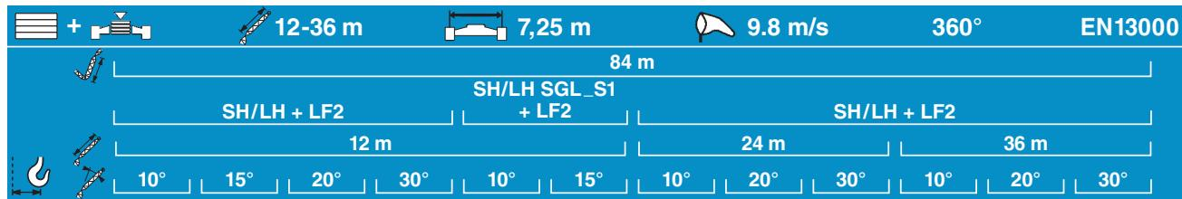
The diagram illustrates the crane's boom configurations. It shows three main boom sections: a long section (12-36 m), a medium section (7,25 m), and a short section (9.8 m/s). The total length is 84 m. The crane is mounted on a turntable with a 360° rotation capability, conforming to EN13000 standards.
