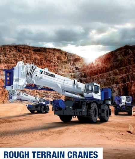
Compact cranes with a single cab for travel and lifting operation. Tadano rough terrain cranes offer ample maneuverability and feature all-wheel steering that enable them to navigate tight work sites. The all-wheel drive means that they are able to travel on rough and uneven terrain without a problem.
