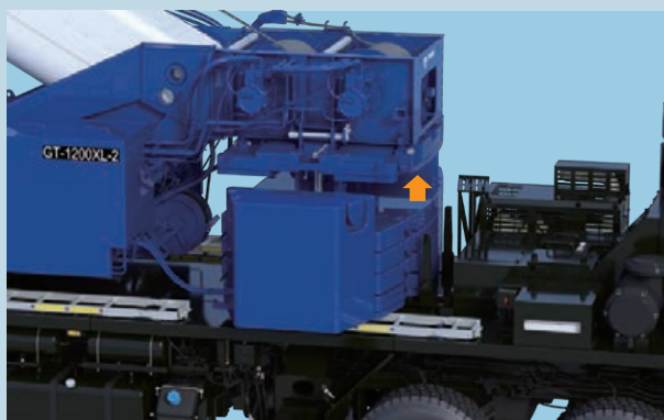
Counterweight mounting/dismounting remote controller
