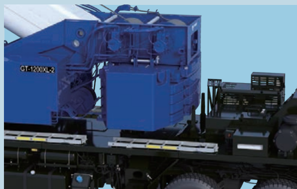
Counterweight mounting/dismounting cylinder
