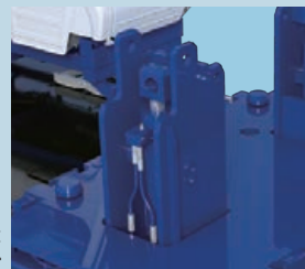
Counterweight mounting/dismounting cylinder
