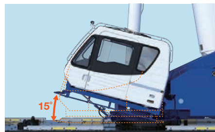
Cab tilt indicator and switch
