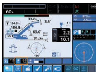
Preset menu display (during crane operation)
