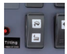
Cab tilt indicator and switch
