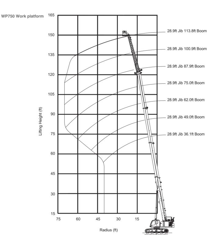
Shaded area is allowable operating range! Limits of operation: Max. load capacity =  $750 \text{ lb} \cdot$
